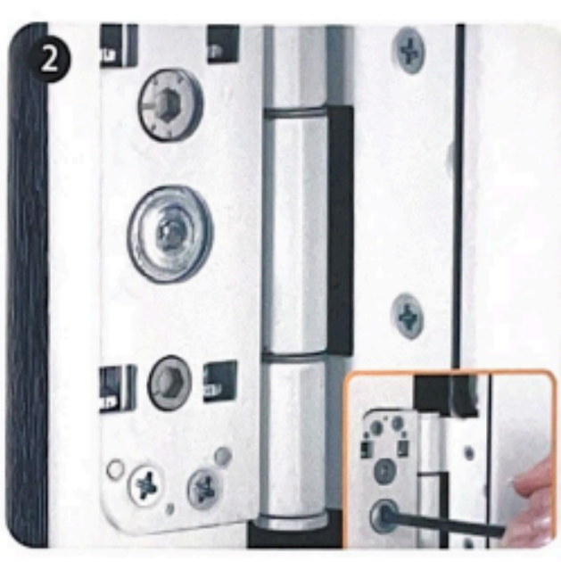
Use a 5mm Allen Key for independent compression, horizontal and lateral adjustments.
